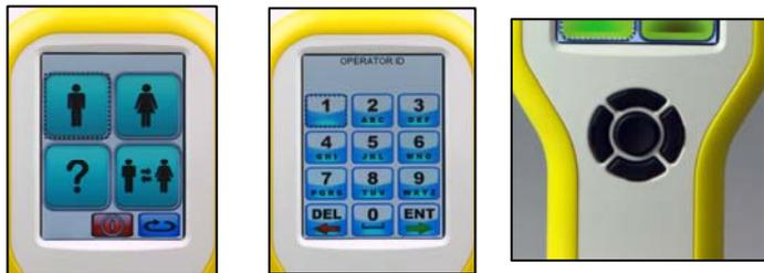
As an alternative to the touch-screen, the five navigation buttons can be used for data entry instead, if required.
