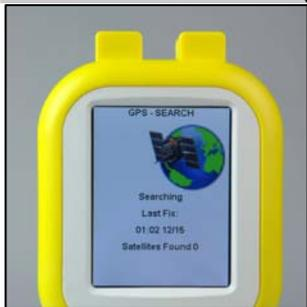
The 600 incorporates an optional GPS system to record the exact location of each breath test - quickly, accurately and fully automatically. These GPS details are stored in memory and can then be transferred to a PC with the actual breath analysis data, where they can then be analysed using standard mapping software.
