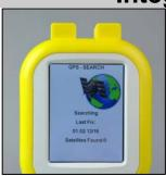
The 600 incorporates an optional GPS system to record the exact location of each breath test quickly, accurately and fully automatically. These GPS details are stored in memory and can then be transferred to a PC with the actual breath analysis data, where they can then be analysed using standard mapping software.
