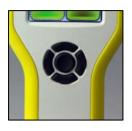
As an alternative to the touch-screen, the five navigation buttons can be used for data entry instead, if required.
