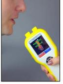
Alternatively, the subject blows into the re-useable sampling cup. In either way, if no alcohol is present the 600 shows PASS - then quickly resets itself, all fully automatically!
