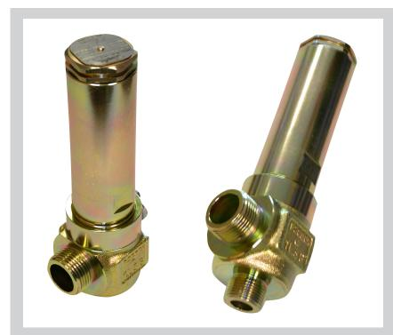
SFA 15 are standard, **back pressure dependent** safety relief valves in angle-way execution, specially designed for protection of vessels and other components against excessive pressure.
