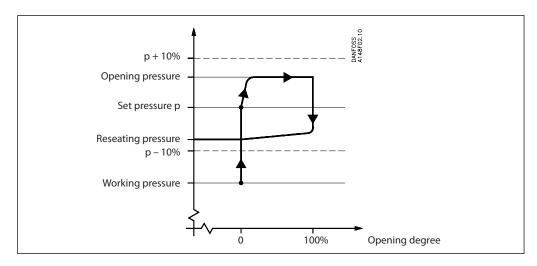
SFA is designed as a **standard safety relief valve** (DIN 3320), which is recommended for refrigeration plants. On a rise in pressure above the set pressure, the safety relief valve will initially start opening slightly, to minimise the outlet of
