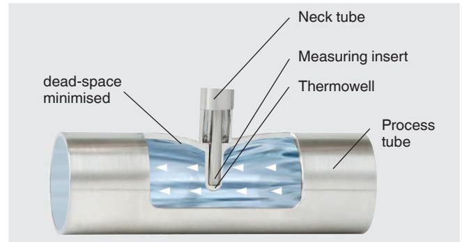
The patented (Patent No. DE 102010037994 and US 12 897.080) hygienic design of the TW61 flow-through housing enables dead-space minimised, invasive temperature measurement and, through self-draining, a flexible mounting position.
