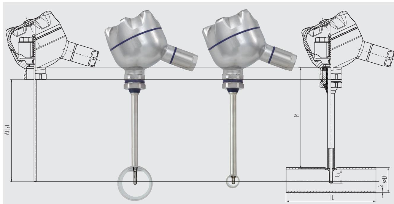
Due to the variable neck tube length M, measuring inserts with standardised insertion lengths A (l<sub>1</sub>) can be used. Thus, variance and stocking of spare parts are minimised. At the same time, the use of correct insertion lengths in the event of replacement is ensured.
