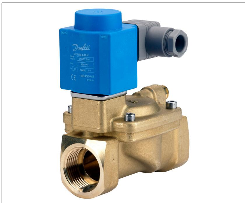
EV224B for compressed air, is a high pressure indirect servo-operated 2/2-way solenoid valve with working pressure up to 40 bar, medium temperature up to 60 °C and available in NC and NO versions.
