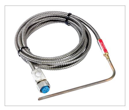
The MBT 5111 is a heavy-duty temperature sensor that can be used for measuring and regulating exhaust gas from diesel engines, turbines and compressors within stationary and marine applications.
