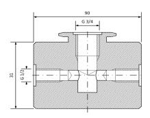
To allow an easy installation into a standard G 1/2 inch line CMT does provide an optional mechanical housing for the sensor.
