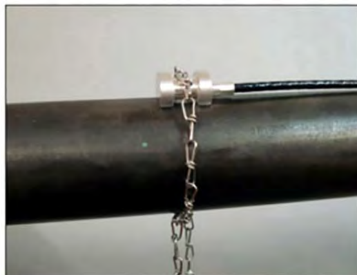
PT100 sensor fixed to pipe
