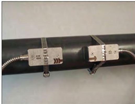
Transducers mounted using strap and clamps
