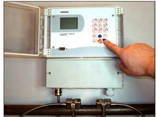
UFM-70 FS wa/1-mounted with transducers
