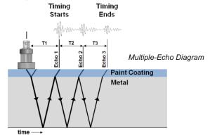
With Multiple-Echo, readings are taken by measuring the time delay between any three consecutive backwall echos. The time of T1 (coating thickness) is ignored. The times of T2 and T3 are equal to the time that it takes to travel through the metal. Only by looking at three echoes can the measurements be automatically verified (where T2 = T3).
