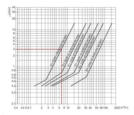
Example, air: Capacity for EV220B 15B at inlet pressure ( $p^1$ ) of 5 bar and outlet pressure ( $p^1$ ) of 3.5 bar: Approx. 245 Nm³/h
