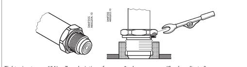
Tightening torque 60 Nm. Zero deviation of approx. 3 mbar can occur. (Can be adjusted)
