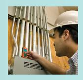
The easy-to-use DT300 Laser Distance Meter accurately measures from 2" to 197' (0.05 to 60m) and can calculate area and volume. The integrated Pythagoras theorem also allows for the user to take indirect measurements. Other features include continuous measurement function with Min/Max distance tracking updates every 0.5 seconds, addition/subtraction, and front or rear edge reference. The DT300 has a double molded housing (IP54), low battery indicator, and auto power-off function.
