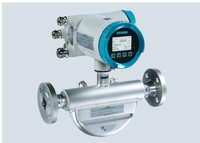
The complete flowmeter system SITRANS FC consist of a new FCS400 sensor in sizes DN 15 to DN 50 mm and a FCT030 multichannel/multifunctional in compact or remote versions. The flowmeter is based on the latest developments within digital signal processing technology – engineered for high measuring performance:
