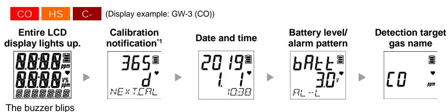
The buzzer blips once, and the power turns on.
