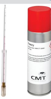
The wax-like solidification of fuel when exposed to low temperatures determines its temperature usability boundary. The relevant indicator for that is the CFPP (Cold Filter Plugging Point).
