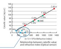
"Opt-Sonic calculation" using measuring results of the Optical sensor and Sonic sensor can minimize the interference effects caused by interference gases, and realize a high-accuracy measurement.
